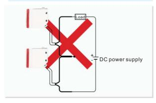
The residual voltage of the sensor is 4V. Before connecting to a relay, be aware of the actuation voltage of the relay.
