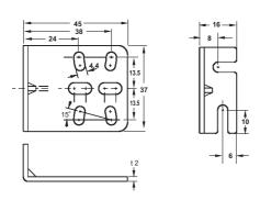
Material: Cold rolled carbon steel(spcc)
