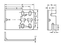
Material: Cold rolled carbon steel(spcc)Two M4(length 16mm) hesagon-socket-head bolts are attached.
